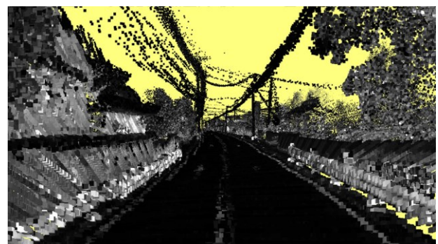
Figure 9. Integrated point clouds (road area)
